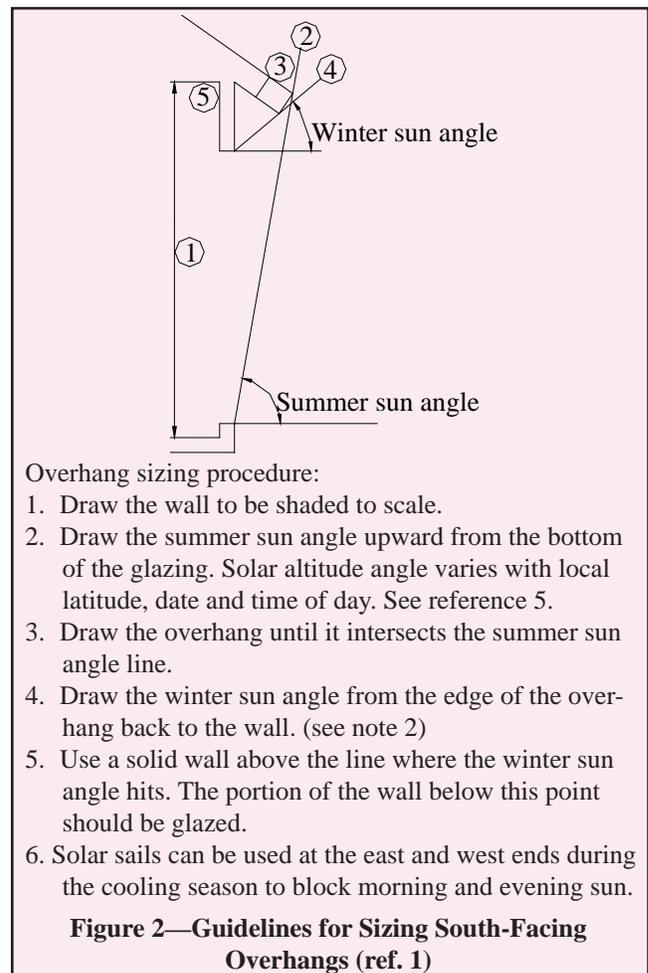
9. **Use appropriate window shading.** Windows facing within about 30° of true south can be shaded with properly sized overhangs. Figure 2 shows guidelines for sizing the overhangs to allow sunlight entry from about mid-September through mid-March (software is also available for sizing overhangs). Off-south wall orientations reduce overhang effectiveness.
