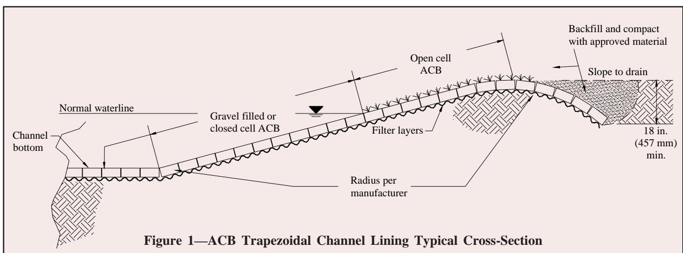
Figure 1—ACB Trapezoidal Channel Lining Typical Cross-Section
