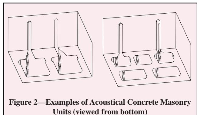
Figure 2—Examples of Acoustical Concrete Masonry Units (viewed from bottom)
