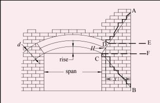
Figure 5—Supporting Adjacent Masonry Must Resist the Horizontal Thrust of the Arch
