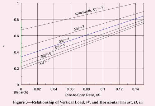
**Small Concrete Masonry Arches**
