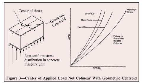
applied load other than at the centroid can provide an array of reported values, Figure 3. Loads not applied through the center of mass of the unit results in lower tested strengths and increased variability in results.
