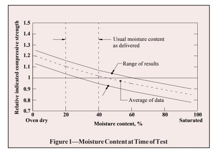
in their "as-received" or "as-desired" moisture condition. To help ensure this, ASTM C 140 requires that units be stored until tested in air at a temperature of 75 + 15 °F (24 + 8 °C) and a relative humidity of less than 80%, and not be subject to oven drying.
