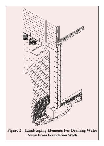
Drainage pipes may also be placed beneath the slab and connected to a sump. In some cases, pipes are cast in or placed on top of concrete footings at six to eight feet (1.8 to 2.4 m) on center to help drain water from the exterior side of the foundation wall.
