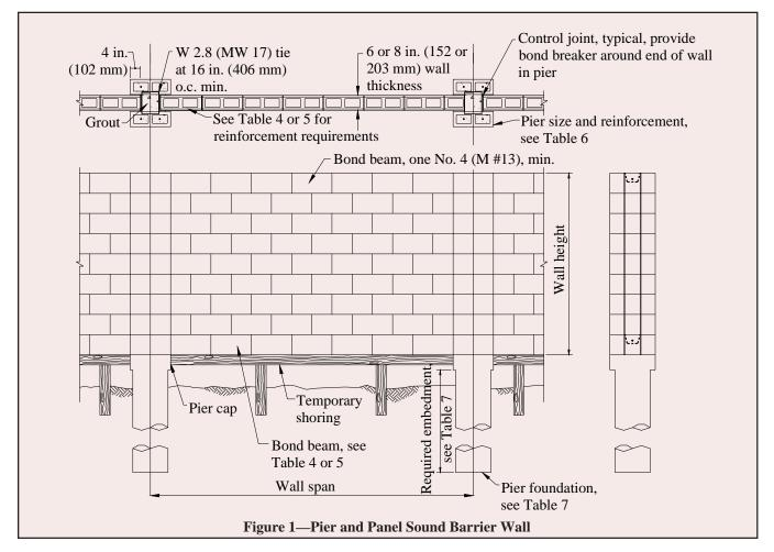
(203 mm) of the wall ends, and at 10 ft (3.0 m) on center along the length of the wall; minimum horizontal reinforcement requirements are satisfied by the primary reinforcement listed in Tables 4 and 5. In SDC D, E and F, vertical No. 4 (M #13) bars are located within 8 in. (203 mm) of the wall ends, and at 4 ft (1.22 m) on center along the length of the wall.
